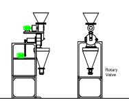
Option C: Micro Pulverizer with Air-Classifier and Dust Collector Discharge - Through Rotary Air-Lock Valve
