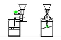
Option B: Micro Pulverizer with Auto-Feeding and Auto-Discharge System Discharge - Through Rotary Air-Lock Valve
